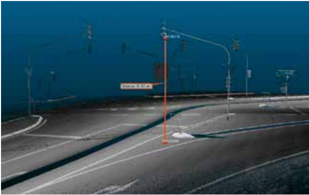
+ Road inventory – 3D position measurement
